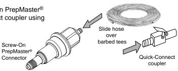
Note: Standard handpiece connections are usually pressure-limited. Use the Quick-Connect to provide higher operational pressure directly from a pressurized gas source. A Hook-up Kit may be required. Ask your local rep or check our web site for kit information at www.GromanInc.com
